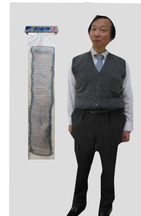
Continuously printed germanium film on an aluminum foil
